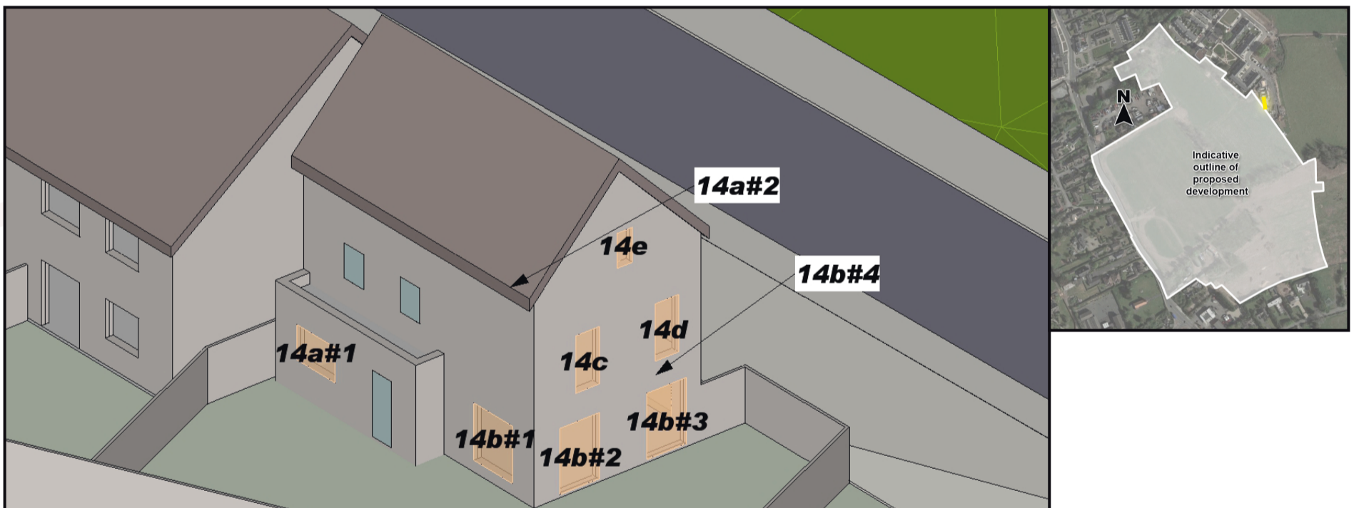
Figure 6.7: (L) - Highlighted areas indicate the position of assessed windows, (R) - Aerial view of assessed location
